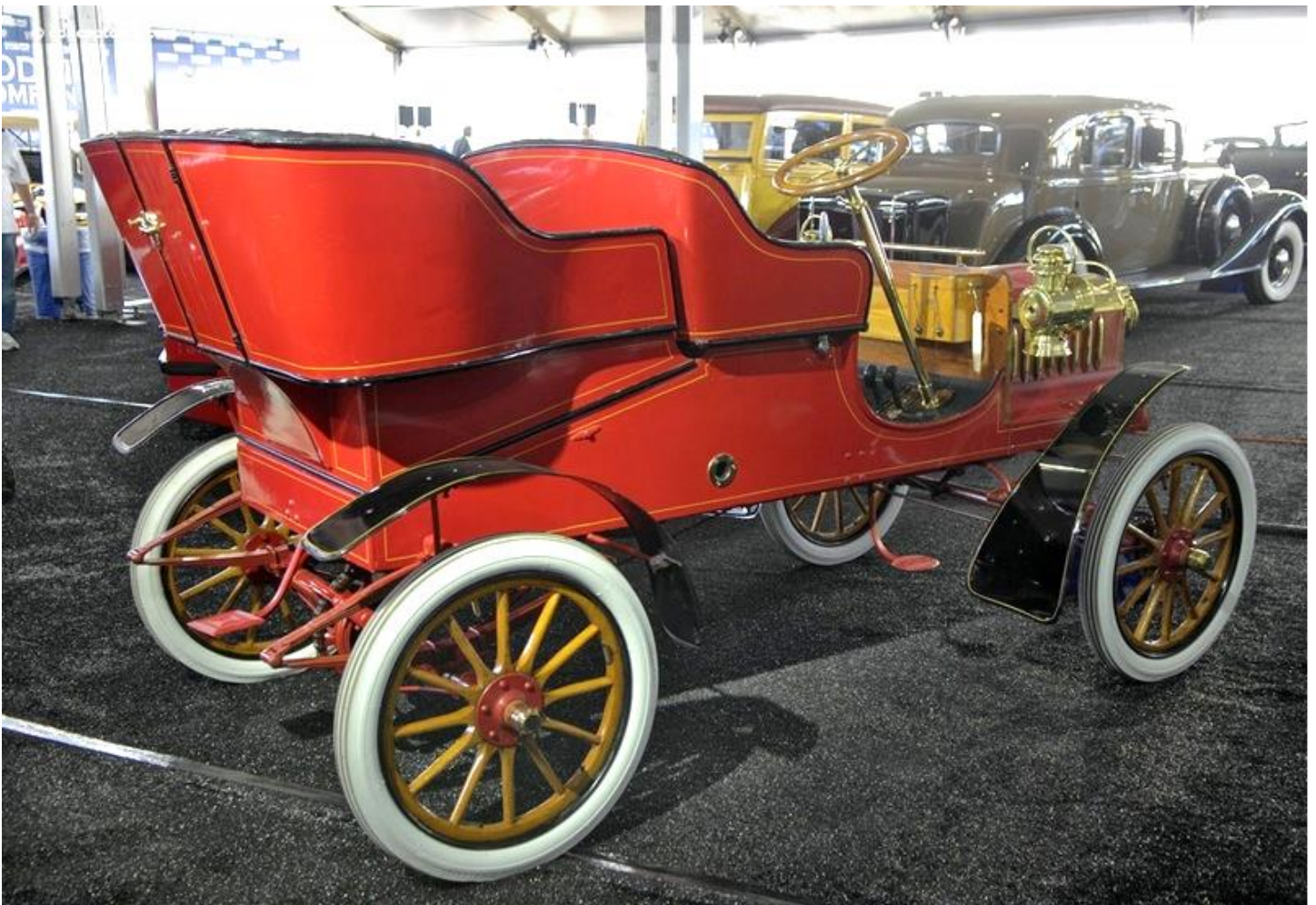
This is a 1904 Model C Touring Car -rear view. Note the rear entrance.
